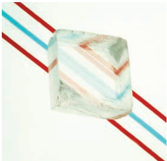
Figure 5 Some forms of the mineral calcite exhibit double refraction when light rays enter the crystal and split.
