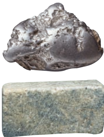
Figure 2 All minerals have either a metallic luster, as platinum does (top), or a nonmetallic luster, as talc does (bottom).
