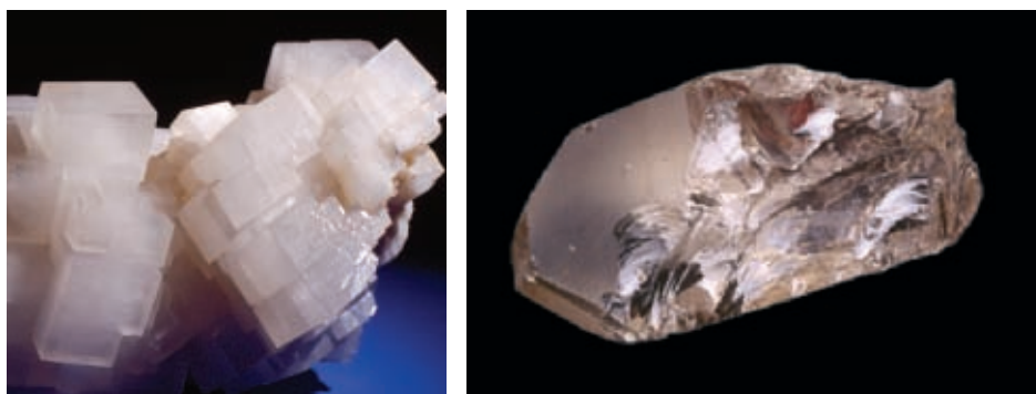
Figure 3 Calcite is a mineral that cleaves in three directions. Quartz (right) tends to have a conchoidal fracture.
